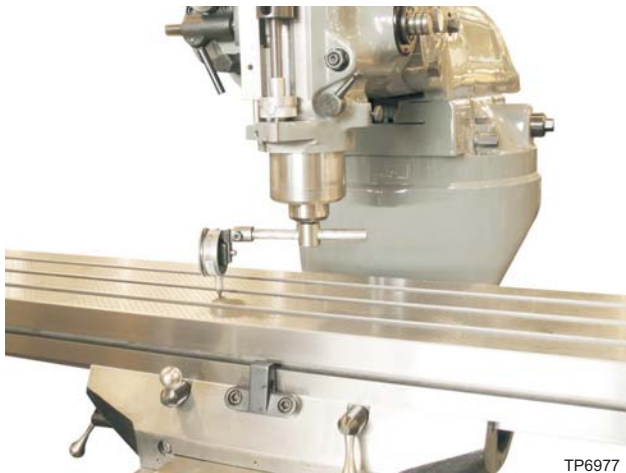
Figure 2.16 - X Tram Check (Indicator to the Left)
