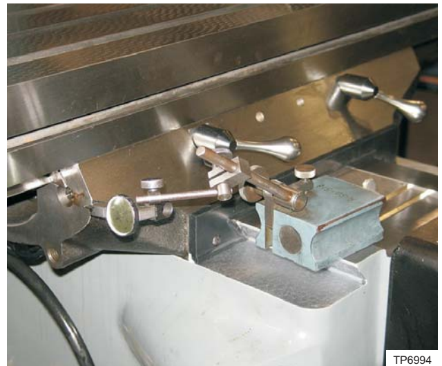
Figure 4.14 - Front Indicator Position for Saddle Gib Adjustment
